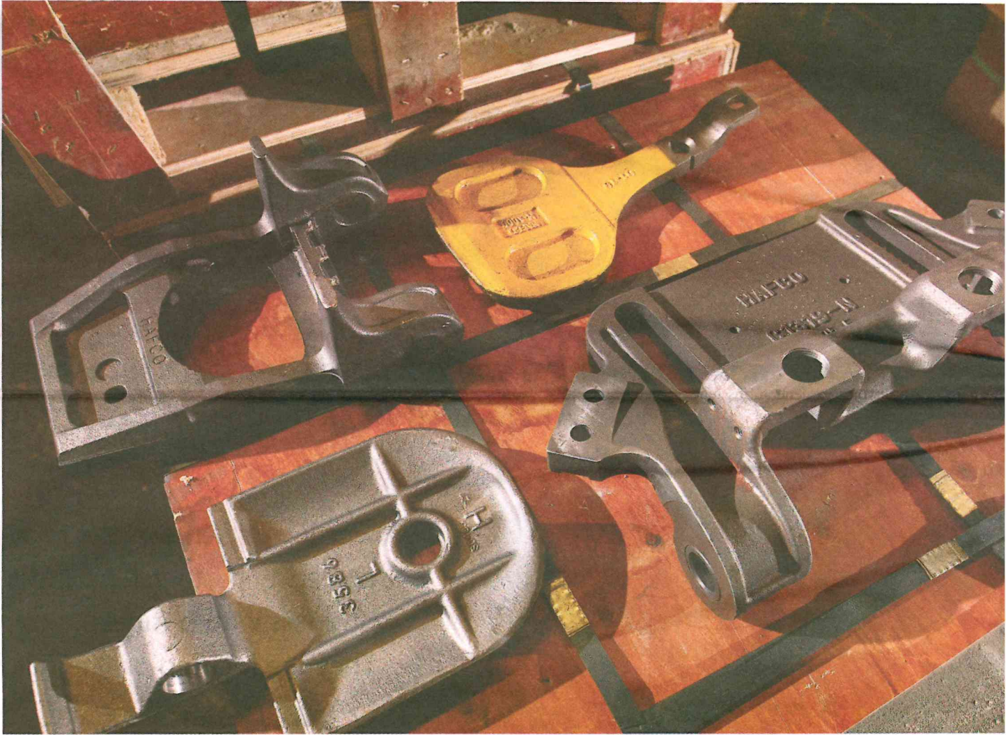
An assortment of castings used in the manufacturing of industrial vacuums made at the Hafco Foundry & Machine Co Inc. — PHOTOS BY ROBERT SCIARRINO
